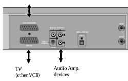
To copy to your player from another video machine, connect the two machines with a cable between their EURO AV (SCART) sockets and select as programme "AV 1/AV 2" or "F. AV" (front sockets) using the [AV], [PR+/-] or [INPUT] button
